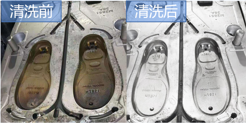
Shoe mold cleaning
